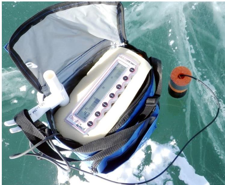
*This is a "Showdown" vertical display sonar rigged for "run and gun" through-the-ice prospecting. The whole unit is in an easy to carry case. If you bring along an insulated container with warm water you can make a quick stop, dribble some water on the ice, set the transducer in the water and get an instant reading of what is below. There appears to be no fishy presence in this shot on 12" of clear hard ice at Starvation.*
