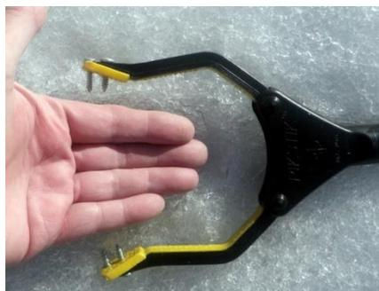
*This is the gripper end of a stronger reach tool. It is wide enough to grab even larger fish. And by adding a couple of screws to the ends you increase holding power for lifting heavy fish by the head or body.*
